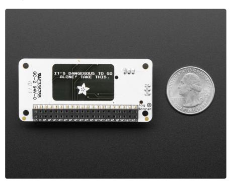
Best of all, this Bonnet is fully assembled - no soldering at all is required. You may need to solder headers onto your Pi Zero (or use press-fit headers) but once that's done you're ready to rock. In theory you could also use this with one of the full-size Pi models, but it wouldn't be very hand-held
