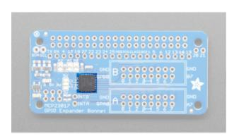
The MCP23017 GPIO expander chip converts Python code into pin instructions.
