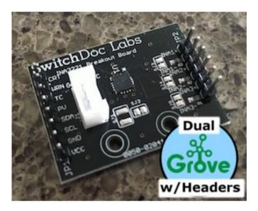
The **Dual Grove/Pin INA3221 Breakout Board** is an easy to use 3 Channel Current / Voltage I2C Monitor.
