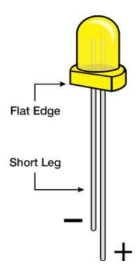
**Note:** It matters how you plug in your LED! Current can only flow in one direction through an LED, so pay careful attention to the leads. The long lead on the LED should be connected on the same row as the  $330\Omega$  resistor.
