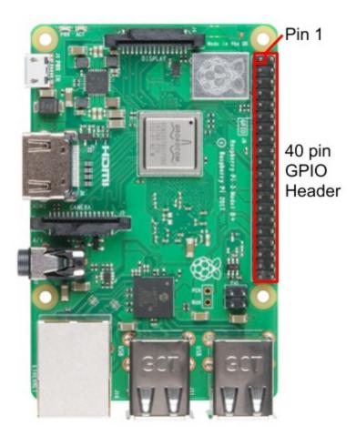
This computer is described in more detail in Source 8. It requires a power supply, HDMI monitor, keyboard and mouse along with the Raspbian Operating System and an Ethernet connection to the Internet. Setting them up is not described in this document.
