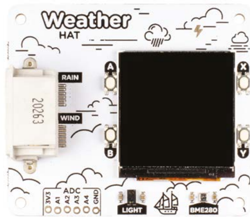
▲ Along with on-board sensors and a mini LCD to show data, the Weather HAT has inputs for wind and rain sensors, plus a breakout header
