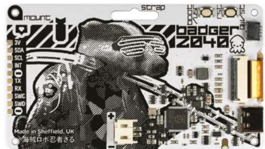
▲ On the rear of Badger 2040 sits the RP2040 chip along with BOOT and RST buttons and a white LED
