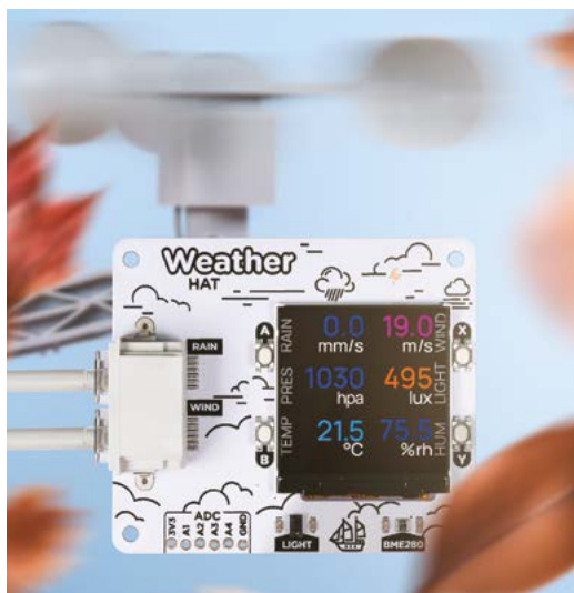
▲ The weather.py Python code example shows live data from the sensors on the LCD
