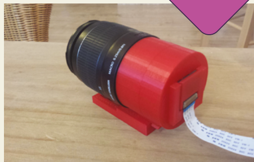
▲ Using a 3D-printed lens adapter, you can use powerful lenses with a standard Raspberry Pi Camera Module
