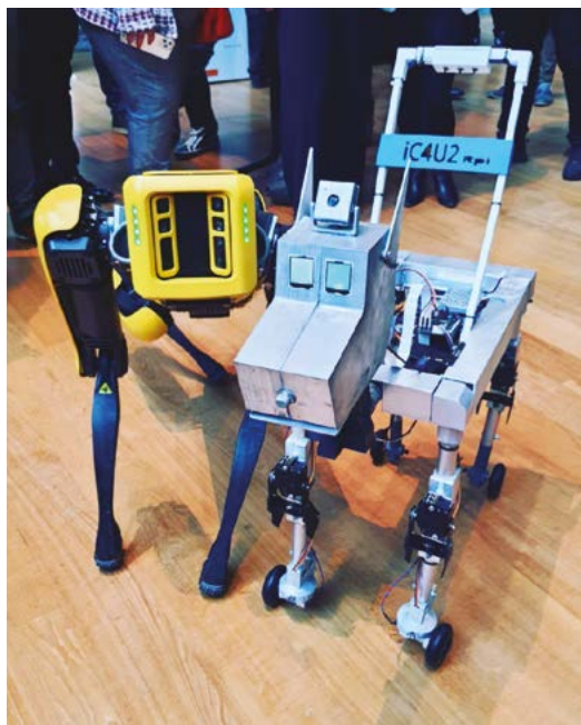
◀ iC4U2 is a Raspberry Pi robot guide dog, one of six robots Selin has designed to date
