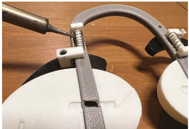
▲ What's behind the eyes? Among the components is a spring from a retractable pen, cut in half
