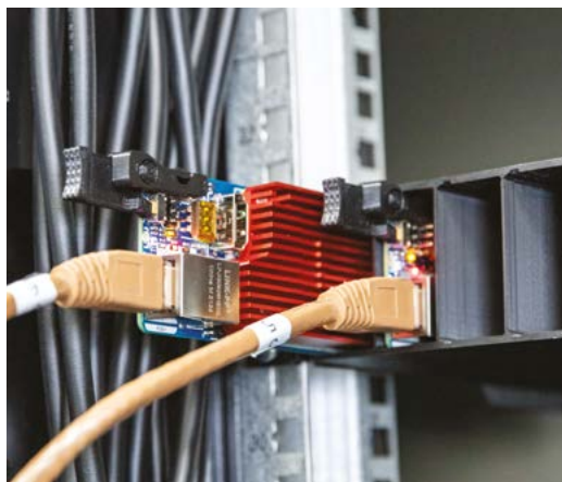
► The two Compute Blade boards we had in for testing mounted in our server rack space
