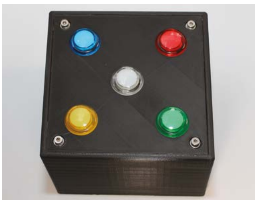
Figure 8 The finished game can be installed into an enclosure. This one is 3D-printed, but you could just use a plastic storage box and drill holes for the buttons
