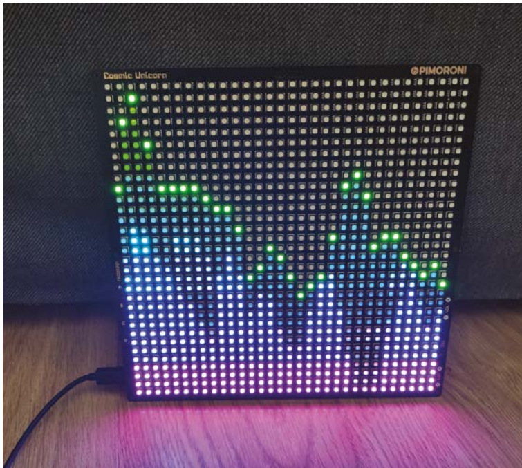
▲ A modified Classic FFT effect on the Cosmic Unicorn, with a greater range of colour and altered offset
