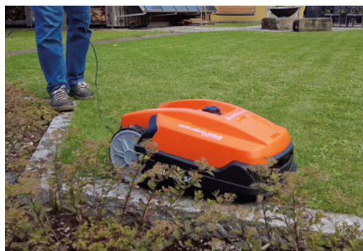
▲ By first driving the robot around the lawn perimeter, and obstacles such as trees, a GPS map is built up for automatic mowing
