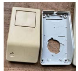
▲ The keyboard and mouse were originally yellowed, but Dan took them apart and used a home-made chemical mixture to whiten them
