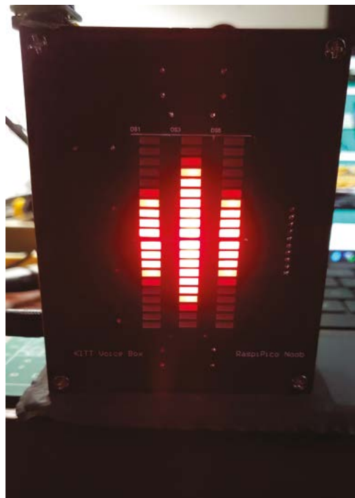
▶ Here's KITT in all his glory! He activates and listens for speech when movement is sensed
