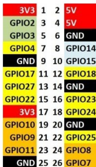
GPIO pinouts for Rev 2 Pi
